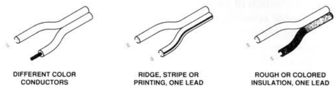
Figure 1: Some Examples Of Polarity Coding On Speaker Cables
