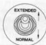
Throw the switch **down** to the NORMAL position if you wish to reduce the current requirement of the woofers. Replace the black cap after setting the switch.
